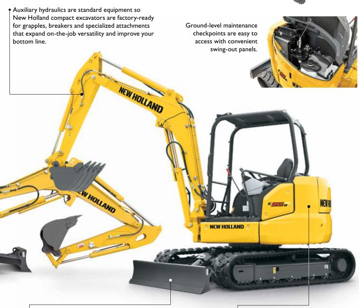
Hydraulically controlled dozer blade is standard to give you added versatility for site prep, backfilling and general grading. The unique blade profile efficiently rolls dirt as it pushes, creating a smooth "wave" of material and creating a smooth, level surface. • New, clean-running Tier 4 Final engines reduce emissions while saving you fuel.
